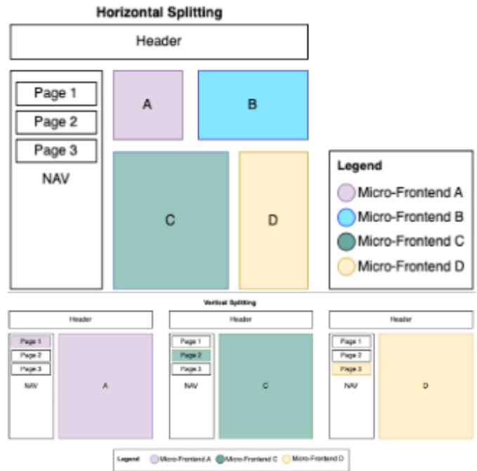
Figure 1: Horizontal vs Vertical splitting
